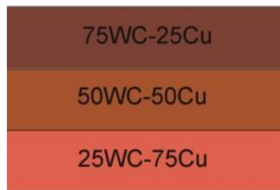
Figure 11 Scheme of the graded composition
