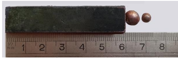
Figure 13 Sample 25WC_bi resulting from hot pressing
