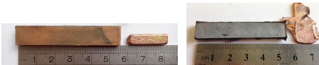
Figure 21 Samples (a) 25WC_mono and (b) 50WC_mono resulting from hot pressing
